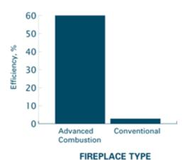
One of the primary reasons for this inefficiency is that large amounts of heated household air flows through the fireplace and up the chimney when a fire is blazing. A conventional wood fireplace will use up to 10 times the amount of air required by a typical oil or gas furnace. And only a small amount of the air drawn into a fireplace is actually used for combustion; the rest, known as excess or "tramp" air, escapes to the outdoors.
