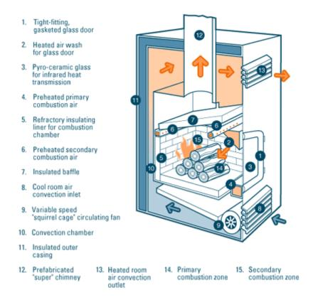
Advanced combustion fireplaces have truly airtight, gasketed doors, a special ceramic (pyro- or neo-) glass window that allows most of the infrared heat from the flame to be transmitted to the room, and a hot air "sweeping" of the window to allow clear viewing. Because these fireplaces are often installed with their back against an exterior wall, they should also have some type of insulated outer casing that prevents unwanted heat loss from escaping.
