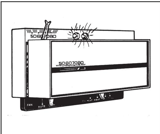
Lights may be used to indicate that the auxiliary electric heat is operating. The lights may be different colors on different types of thermostats. Typical lights will be blue or green for normal auxiliary heating and red for emergency heat.
